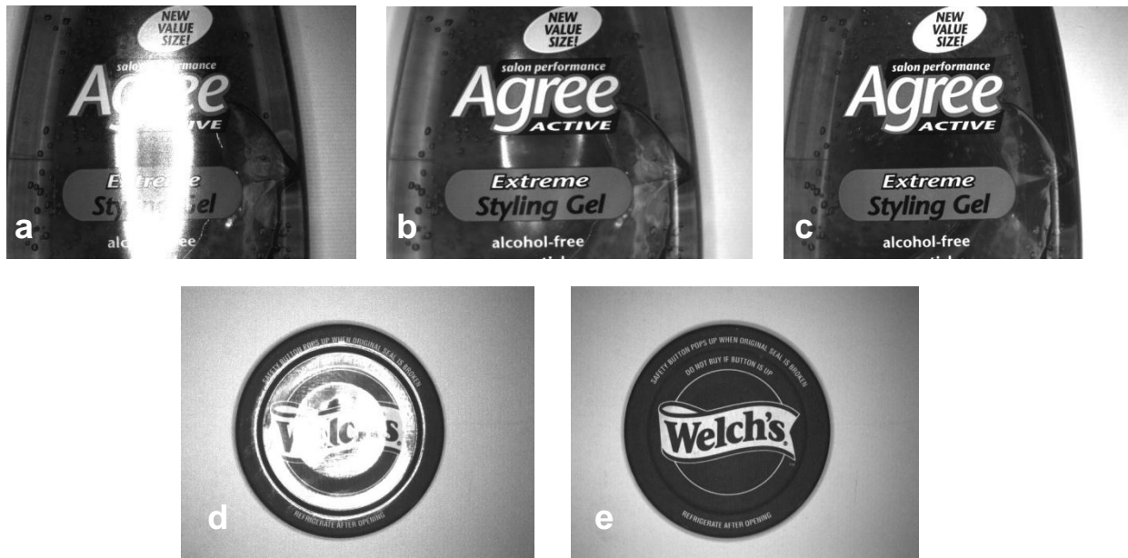
Fig. 18 - A change in “lighting – sample – camera” geometry or type may be more effective than applying polarizers to stop glare. a – Coaxial Ring Light w/o Polarizers. b – Coaxial Ring Light w/ Polarizers (note some residual glare). c – Off-axis (light axis parallel to the sample long axis) Ring Light w/o Polarizers. d – Coaxial Ring Light w/o Polarizers. e – Coaxial Ring Light w/ Polarizers (note: 2 ½ f-stop opening).
