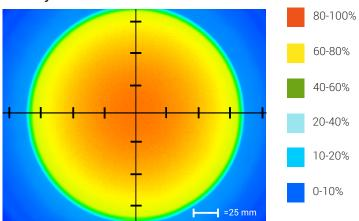
Optical measurement taken using FX0808-WHII3 @ 200mm
