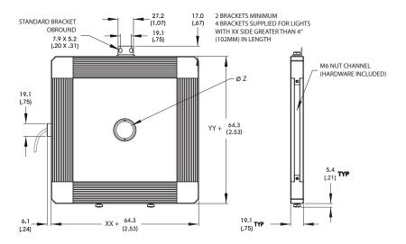
YY = WIDTH IN 1" INCREMENTS FROM 3" to 24" XX = HEIGHT IN 1" INCREMENTS FROM 3" to 24"
